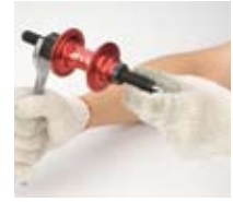
5. Tighten the lock-nut in drive side
