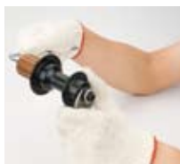
2. Un-tighten the alloy end cap from drive side
