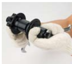
1. Un-tighten the lock-nut by wrench
