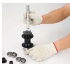
12. Put the axle inside the hub shell
