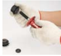
3. Take the 1sp freehub body and slide into the axle
