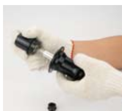
24. Slide the new free-hub body inside the axle
