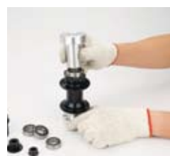
14. Take the holding tool(C) onto the bearing (disc side)
