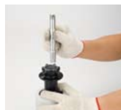
9. Put the axle inside the hub shell from disc side
