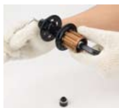
25. Tighten the alloy end cap(non-drive side) with force 100kgf.cm by allen key
