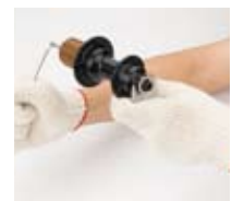
6. Tighten the lock-nut in drive side
