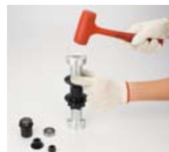
19. Install the bearing with rubber hammer
