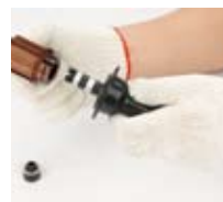
4. Slide in the new freehub body
