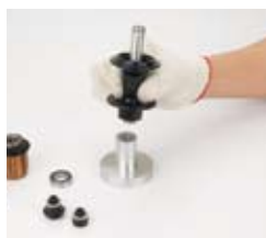
16. Put down the hub(non-drive side) on holding tool(C)
