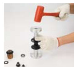
15. Install the bearing with rubber hammer
