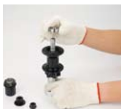
20. Take the other bearing for drive side
