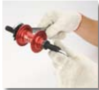
1. Un-tighten the lock-nut from drive side
