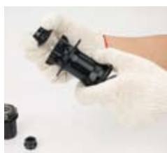
22. Threaded the alloy end cap(disc side) onto axle
