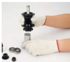
16. Put down the hub on holding tool(C)
