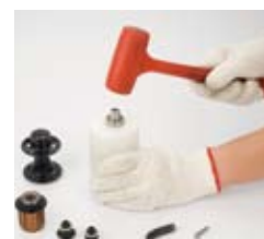
10. Push out the bearing from the axle by rubber hammer
