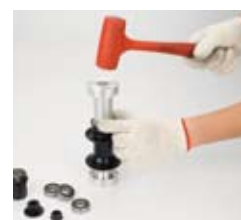
15. Install the bearing with rubber hammer
