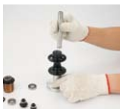
12. Put the axle inside the hub shell
