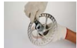
5. Tighten up lock-ring with torque of 400 kgf.cm
