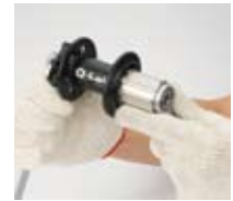
6. Tighten the lock-nut in drive side
