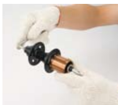
1. Un-tighten lock-nut from non-drive side
