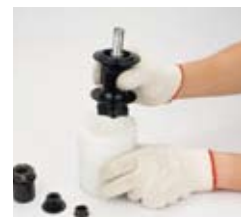
5. Put down the hub(disc side) on holding tool(A)
