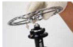
3. Assembly 2 in one then put it onto KT Q-LOCK disc hub mount
