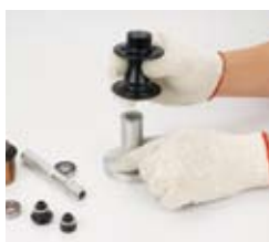
11. Put the hub shell onto holding tool(B)
