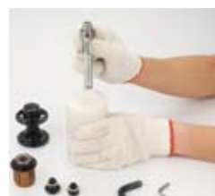
9. Put the axle down to the holding tool(A)
