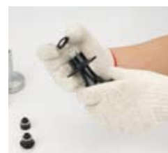
23. Take the seal and push it into hub shell (non drive side)
