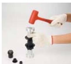
21. Take the holding tool(B) onto the bearing (drive side)
