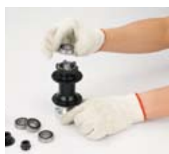
13. Take on bearing onto hub shell(disc side)
