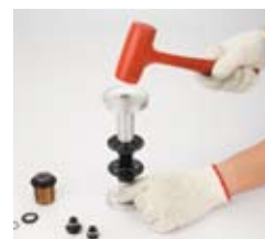
19. Install the bearing with rubber hammer
