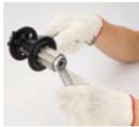
2. Un-tighten the lock-nut in drive side
