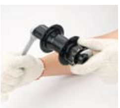
25. Threaded the lock-nut (drive side)
