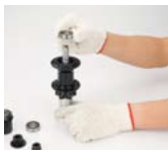
17. Take one bearing on the axle(drive side)
