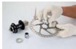
2. Take patent adaptor and put it into rotor 6 holes
