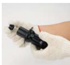
26. Tighten the lock-nut(drive side) with wrench
