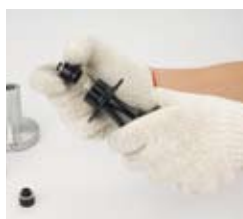
24. Threaded the end nut from non-drive side
