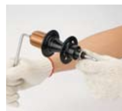
27. Tighten the alloy end caps in drive side with force 120kgf.cm by allen key
