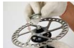
4. Take lock-ring and screw into Q-LOCK disc hub
