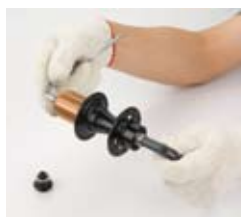
3. Un-tighten lock-nut from drive side
