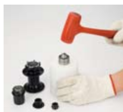
8. Push out the bearing by rubber hammer
