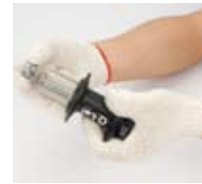
5. Threaded the lock-nut in drive side
