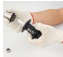
4. Slide in the new freehub body
