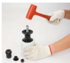
6. Push out the bearing by rubber hammer
