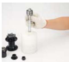
7. Put down the axle & bearing to holding tool(A)
