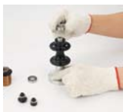
13. Put the bearing on non-drive side
