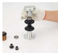
14. Put the holding tool (C) onto the bearing
