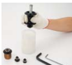
6. Put down the hub on holding tool(A)
